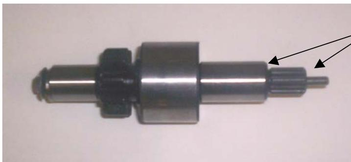
Remove material from these two surfaces as required to meet air gap of .075" - .125"
